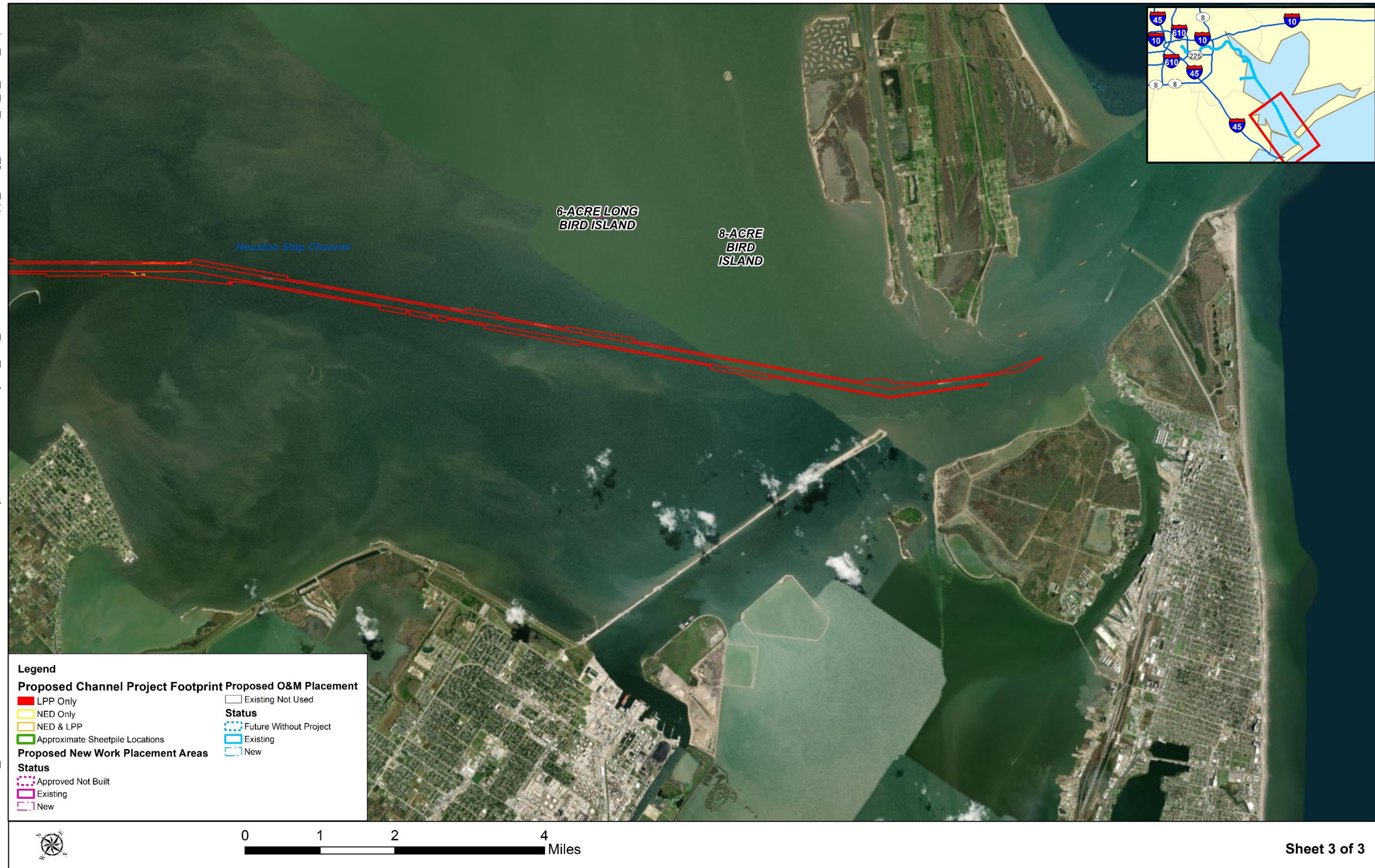
Figure G3.2-3 Proposed Channel Project Footprints and New Work and O&M Placement Areas for the NED Plan and LPP – Sheet 3
